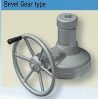
BGA series are bevel gear actuators that can be attached directly to gate and globe valves that are subjected to thrust, realizing easy manual operations. By using an adaptor, the actuators can be easily attached to existing valves. In addition to the standard type, BGA series includes BGA-P type with a position indicator, BGA-S type with a limit switch, and BGA-W type with two orthogonal shafts.
