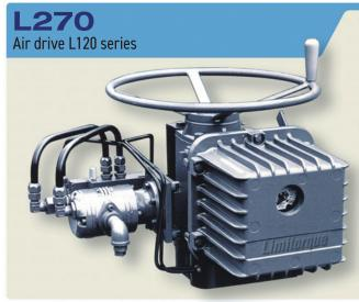
Similarly to the pneumatic type of SMB series, L270 series can be operated by using compressed air as the power source. The internal gear transmission mechanism is the same as that of L120 series. Air micro switches are used for the limit and torque switches, and those operate pilot valves and control the actuator. It is also available to attach electric equipment for L120 to the actuator with only the motor being pneumatic.
