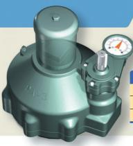
PA series are actuators developed for water gate valves, and equipped with a spur gear. The actuators have a compact design with a built-in thrust bearing. Similarly to BA series, by using an adaptor, they can be easily attached to existing valves. In addition to the standard type, we also offer PA-P type with a position indicator and PA-S type with a limit switch.
