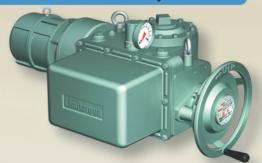
Small-sized JMB-04 and 03 have a declutch lever, and medium-sized JMB-00 to large-sized JMB-4 have a push-pull handle. For all models, manual/electric switching can be done with one-touch operation. The actuators are equipped with an interlocking switch which shuts off electric currents during manual operations. They can be used for various purposes, including sluice valves, globe valves and water gates.
