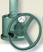
B series are bevel gear actuators for manual operations. By combining two B series actuators with an SMB series actuator, they can be used for opening/closing a double-spindle gate. Dimensions of the unit's mounting surface and stem are the same as those of SMB series. Accordingly, in case of the need for converting to an electric actuator, B series can be easily replaced with SMB series. Models with a position indicator are also available.
