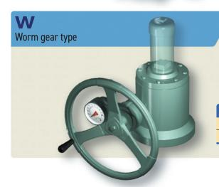
W series are worm gear reducers for manual operations. Similarly to B series, dimensions of the unit's mounting surface and stem are exactly the same as those of SMB series. Accordingly, W series can be easily replaced with SMB series electric actuators. Worm and worm gear set of W series are the same as those of SMB series, and various models with different gear ratios are available. Models with a position indicator are also available.
