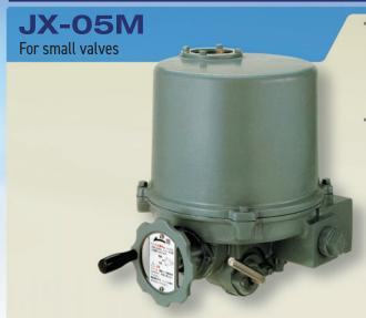
Super small JX-05M series are electric actuators developed for small globe valves and small gate valves. Making use of our wealth of long experience as a pioneer of valve actuators, we designed this series to meet customers' demands. As a result of pursuing usability and safety, a hand wheel is included as a standard feature, and the automatic return mechanism is adopted for manual/electric switching.
